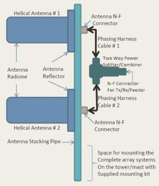
Dual Stacked Helical Antenna Schematic Diagram
